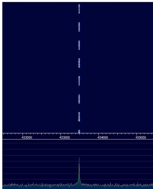
Figure 5.1: Beacon signal seen on a Spectrum analyzer with waterfall
